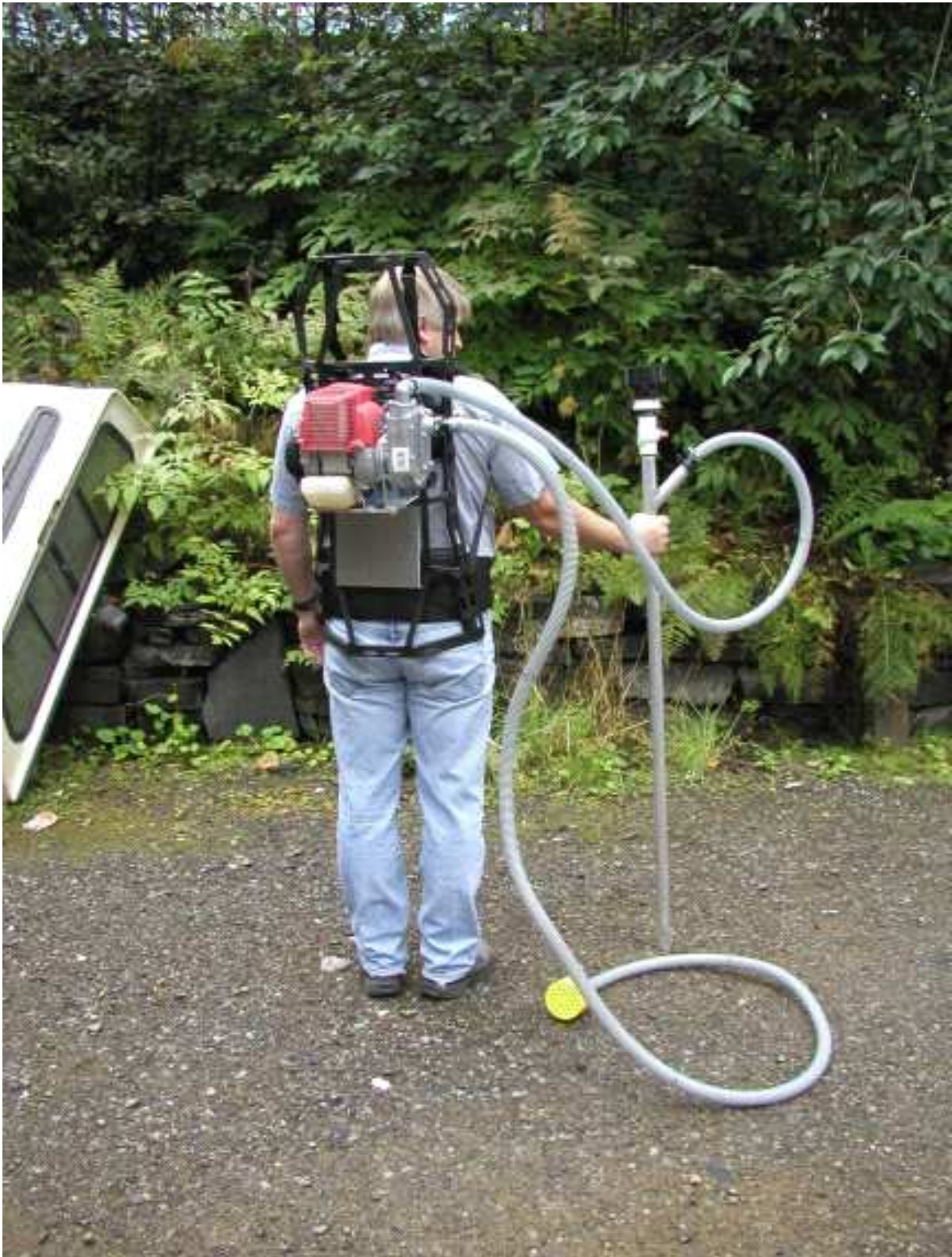
Figure 4. Picture showing the hydraulic egg planting device.
