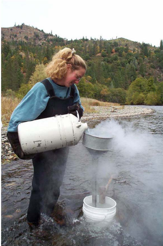
Figure 9. Photograph of the freeze-coring process; liquid nitrogen is being poured into a standpipe to freeze a sample of the substrate. (from Evenson, 2001)
