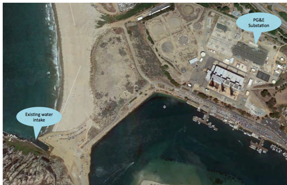
Figure 1 - MBO Export Cable will use the Existing Discharge and connect to the PG&E Substation
